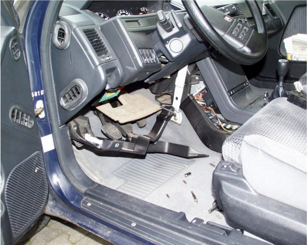
Fig. 1 : Panel under the steering wheel and carpet covered panel removed.
