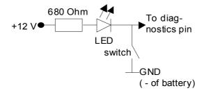
In case the large 30 pins diagnostic connector is present only a wire to connect the diagnostic pin to ground is needed. The readout will work via the diagnostic lights on the dashboard. (In case it doesn't work, one can always revert back to the circuit described above.)
